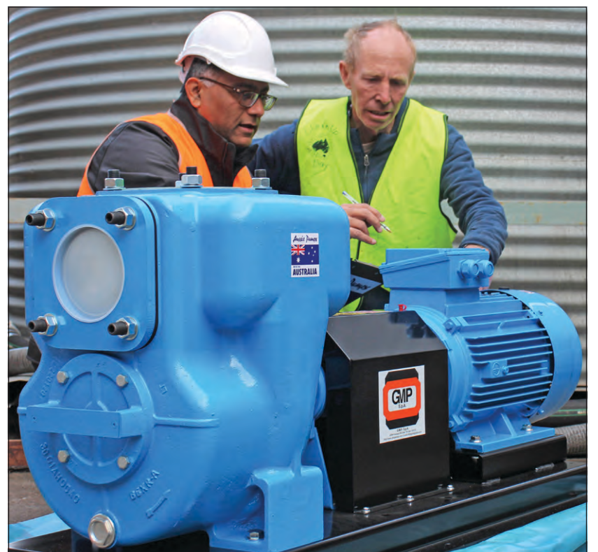
This big 6" 4000LPM self-priming pump will soon come with a 316 stainless-steel impeller.
