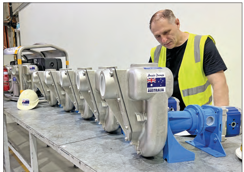
Aussie Pumps new 4" 316 stainless-steel pump in hydraulic-drive configuration.
