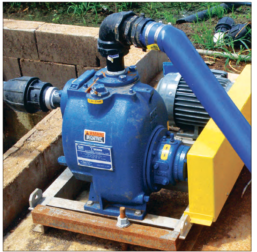
The Gorman-Rupp T2A3-B is a rugged self-priming centrifugal solids-handling pump.
