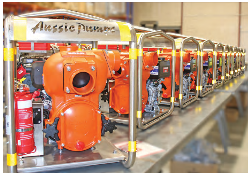
Aussie 4" trash pumps are designed to handle effluent.
