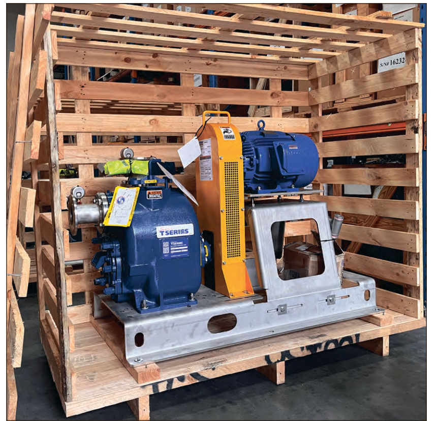
A Gorman-Rupp T3A71S-B pump with hardened internals was selected for the harsh environment of the refinery's recovery pit.
