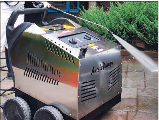
The Aussie Sizzler delivers 80C at 1800psi. Used with a turbo, it's effective working pressure is 3100psi. All this from a 240V 2.7kW single-phase motor.
