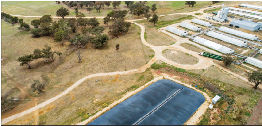
Blantyre Farms uses digester dams to capture methane which is converted into electricity.
