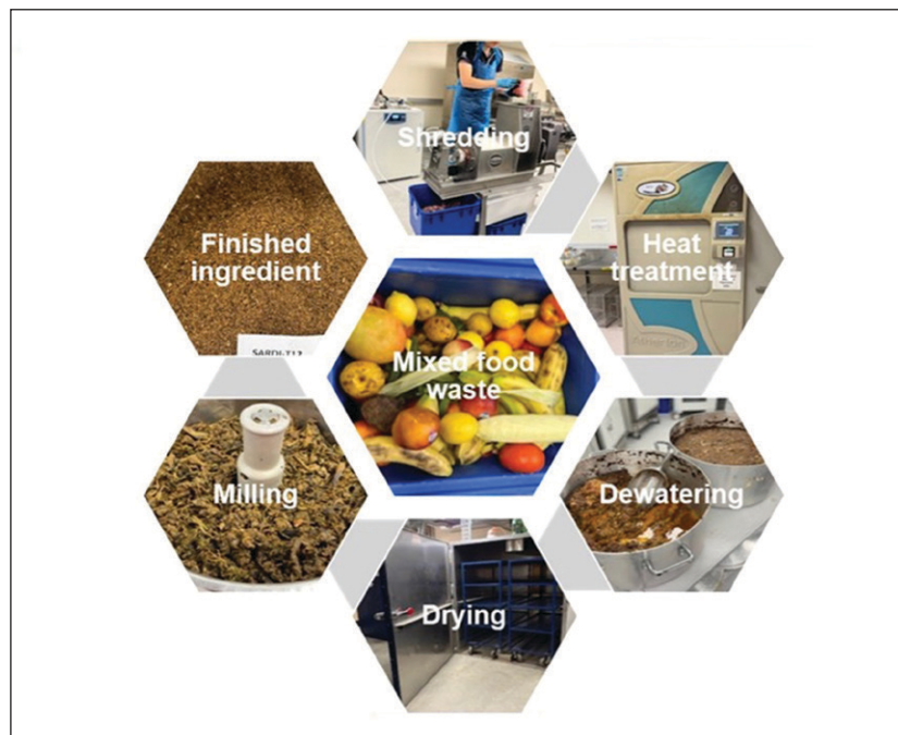
Figure 1: Process of treating mixed food waste into a dry feed ingredient. The material was initially macerated/shredded and then heat treated, dewatered, dried and milled into a feed ingredient.
